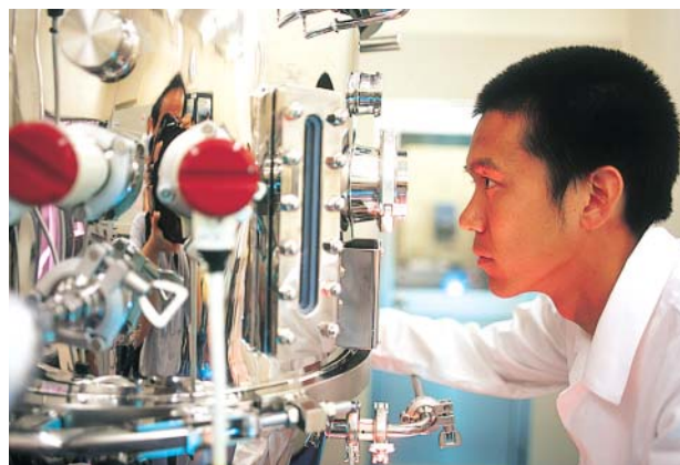
This pharmaceutical spray dryer processes a continuous, sterile stream of solutions, suspensions or emulsions into powder, contributing to substantial reductions in time and costs.
