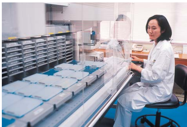
The Genesis Workstation operates a robot that automatically retrieves compounds that have been selected from a library of several hundred thousand compounds.
